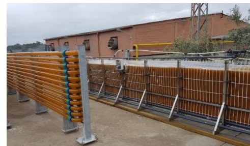
Figure 5-2: Closed flat-panel GW photobioreactors from A4F growing carotene-rich Dunaliella at the Monzón Biotech production unit in Spain.
