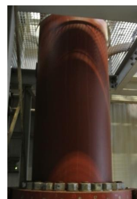
Figure 5-5: Industrial plant HD12 for scCO 2 -extraction of algae biomass at NATECO
